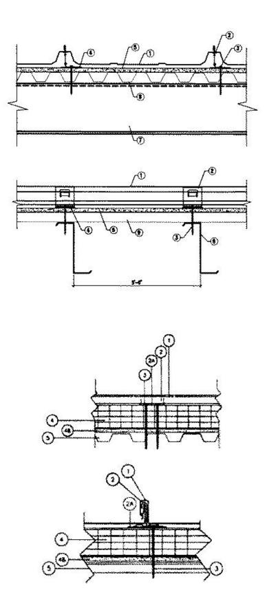
1. Metal Roof Deck Panels\* — No. 24 MSG min. Coated steel panels continuous over two or more spans. End laps to occur adjacent to purlins with panels overlapped 3 inch max. Side laps to be tightened and crimped with a special
